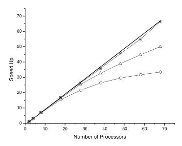
Speedup (calculated as length of time for calculation on a single processor / length of time for calculation on n processors) for docking a library of 500 different small molecules (circle), 1000 different small molecules (triangle), and 1000 copies of nevaripine (star) using flexible ligand docking as a function of the number of processors in MPI mode. A perfectly parallel calculation (bold line) is plotted for comparison.
